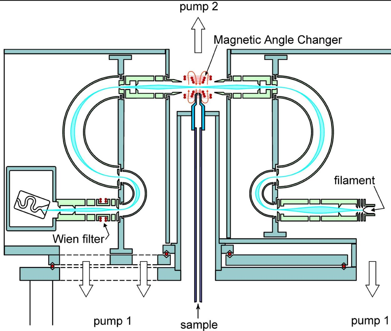
The "Magnetic Angle Changer" (MAC), developed by Reid and Channing, makes it possible to measure the full angular range, including  $0^\circ$  and  $180^\circ$ .
