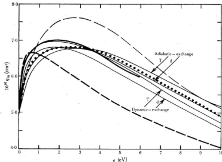
Fig. 7.—A comparison between theoretical and experimental momentum transfer cross sections. — Crompton, Elford, and Jory; - - Frost and Phelps; - · - Bauer and Browne; — La Bahn and Callaway; ●●● Williamson and McDowell.
