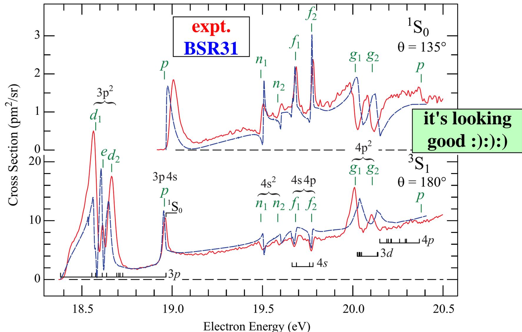
Expanded view of the resonant features in selected cross sections for the excitation of the 3p states. Experiment is shown by the more ragged red line, theory by the smooth blue line. The present experimental energies, labels (using the notation of Buckman *et al.* (1983), and configurations of the resonances are given above the spectra. Threshold energies are indicated below the lower spectrum.
