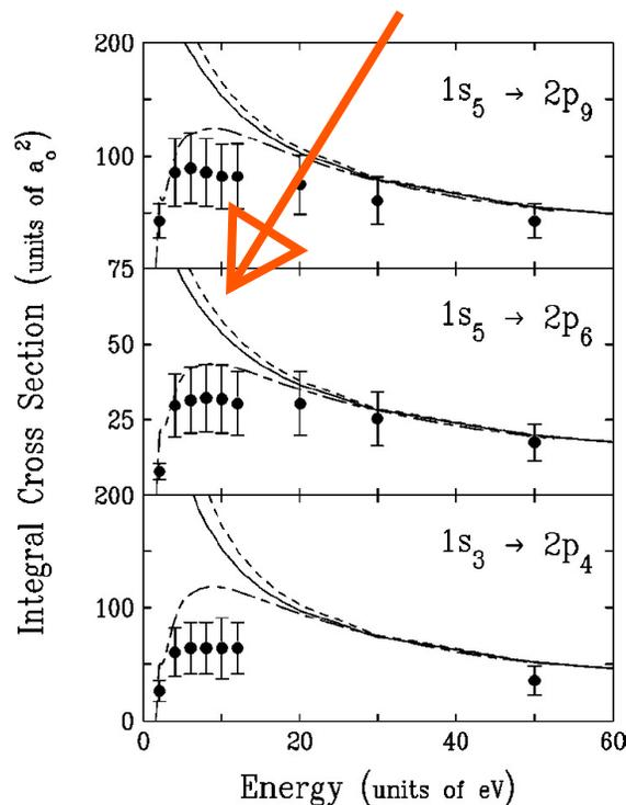
FIG. 2. Integral cross sections for electron-impact excitation of three states in the  $2p$  manifold of argon from the metastable states in the  $1s$  manifold as a function of incident electron energy. The experimental data are those of Boffard *et al.* [7]. The theoretical results are PWBA (dashed curve); 15-state  $R$ -matrix results (long-short dash); and SRDW with CIV3 wave functions (solid curve).
